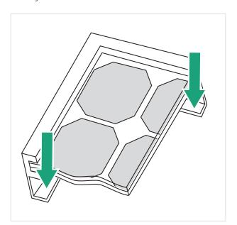
The maximum distance from the roof surface to the mounting profile is 11,5 cm. Is the distance higher? Then use the BB200.
