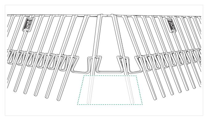
12 Check that the BirdBlocker covers all around and that there are no openings for a bird to pass through.
