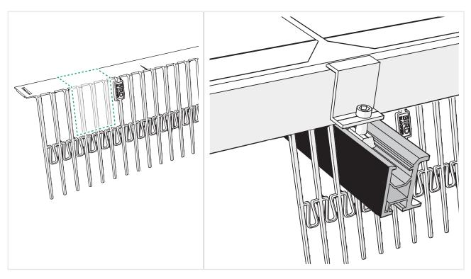
10 Attach the Birdblocker strips to the profiles of the solar panels.
