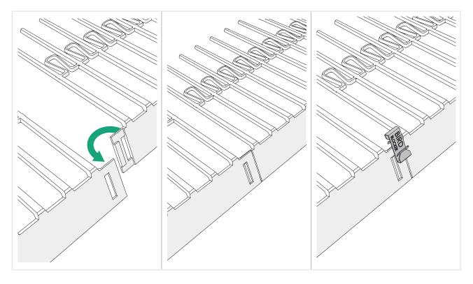
9 Is there a break in the solar profile? Cut a recess in the strip.
