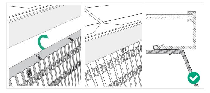
Are the needles of an outer corner under too much tension on the roof surface? Then cut the needles shorter so that they just touch the roof surface.
