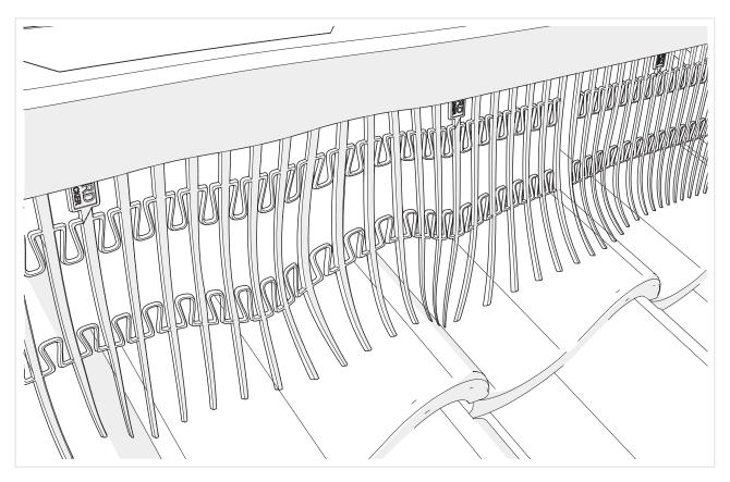
13 Connect the loose strips together with cable ties.
