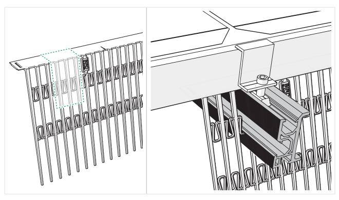
10 Attach the Birdblocker strips to the profiles of the solar panels.
