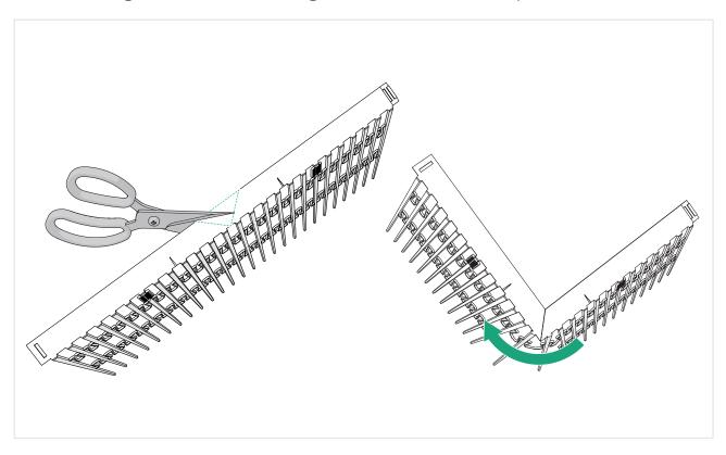
Then prepare the BirdBlocker strips for the inner corner profiles (number of inner corner points **B**). Cut the top of the BirdBlocker edge and fold the BirdBlocker strip outwards.
