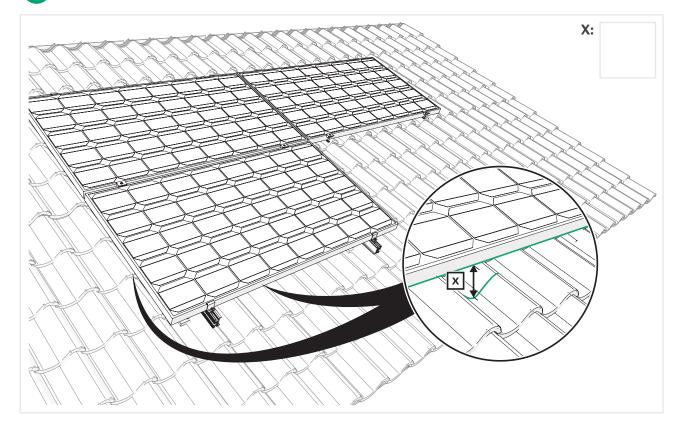
3 Clip test – Take a clip and slide it into the flat part of the profile at the back of the solar panel.
