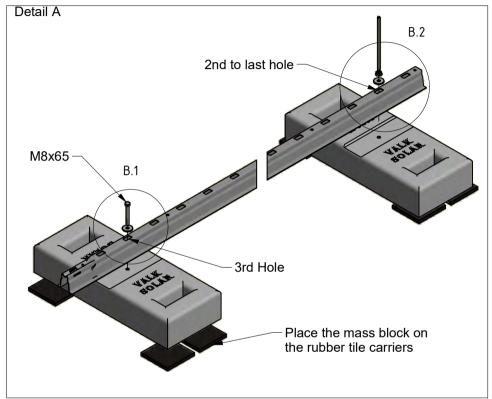
Mount the mass blocks to the roof carriers in the correct positions.
