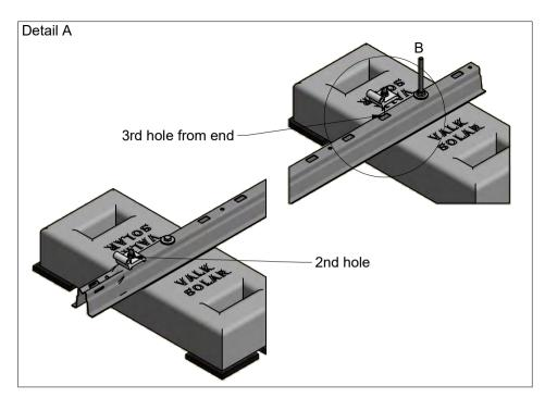
Mount the connector pieces to the roof carriers. Make sure they are placed as shown in the drawing.
