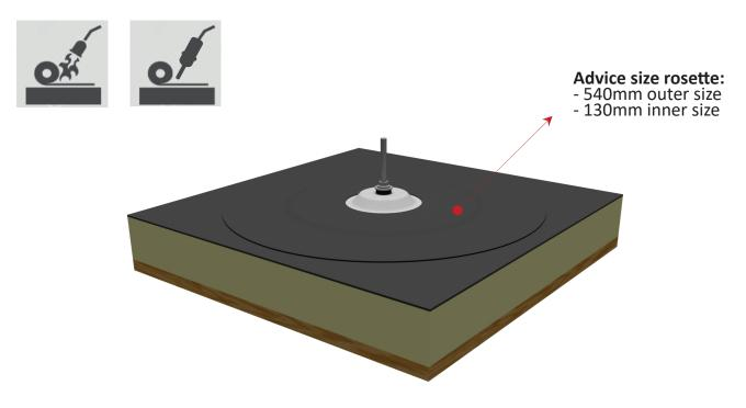
For the watertight finishing of the consoles please contact your certified roofer. Advice: first degrease the ValkSolarFix before making a watertight seal.
