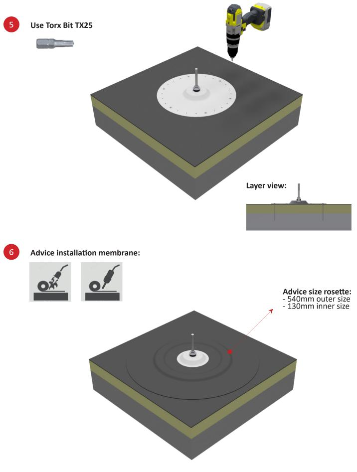
For the watertight finishing of the consoles please contact your certified roofer. Advise: first degrease the ValkSolarFix before making a watertight seal.
