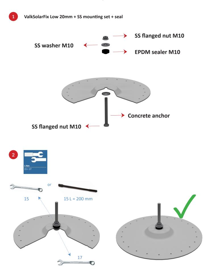
Installation manual ValkSolarFix / Mounting in aerated concrete with aerated concrete screws
