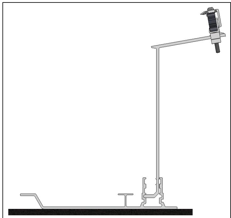
The mounted backfoot can now be placed below the high side of the panel and the clamp can be fixed to the panel frame. The front foot can be fastened to the panel frame on the low side of the panel.
