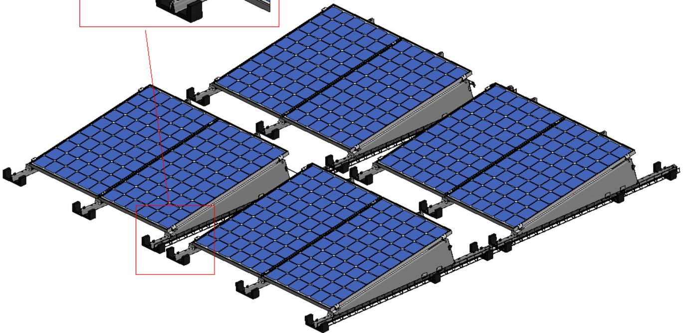
In positions where there is a dilatation in the system, a metal dilatation wire (732020) can be used. This wire can be placed in the cable clamps and the length can absorb the thermal expansion of the coupled system. The electrical cables can be fixed to the wire using tie-wraps. This keeps the cables free from the roof surface.
