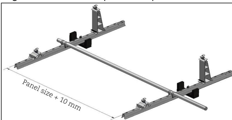
The alignment set can be used to make sure the roof carrier rows are placed at the correct pitch beside each other.
