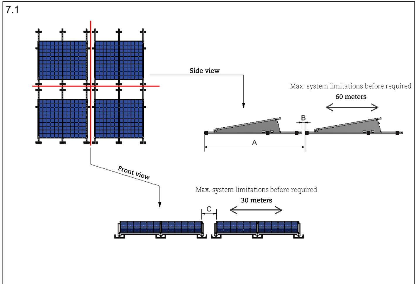
The dimensions below refer to the distance limitations of the dilatation for the outer panels of the system to be 'shielded'. In case these distances are longer, the outer panels of the system, need to be seen as 'exposed', which means more ballast needs to be placed, compared to 'shielded' panels.
