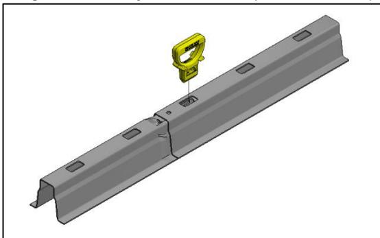
The alignment key can be used to align the overlapping oblong hole of the roof carriers.
