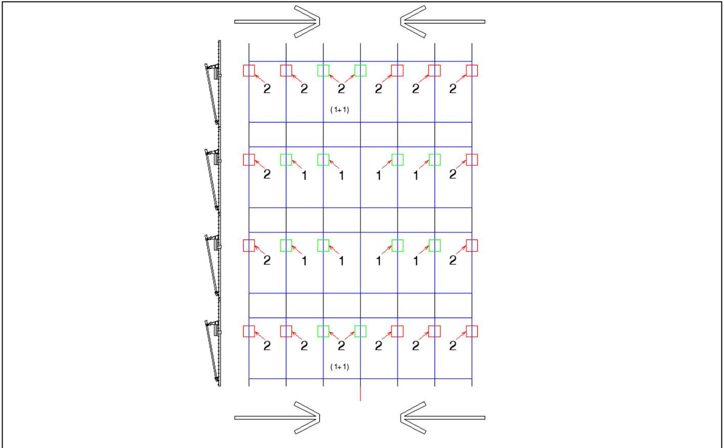
The required number of tiles is indicated per panel (same as the project report). The ballast is always placed starting from the outside toward the centre of the system. Therefore the middle row of the system doesn't have any ballast (see red line). If possible there may be ballast placed on those foundation points as well.
