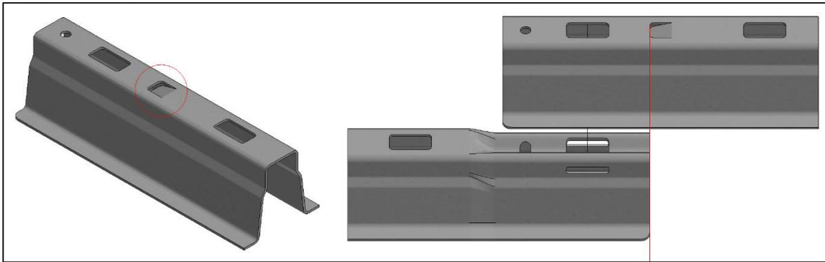
The smooth side of each roof carrier is provided with a lip which can be used when aligning / coupling the roof carriers. The swaged end of the roof carrier can be placed against the lip, this makes sure the roof carriers are always aligned properly.
